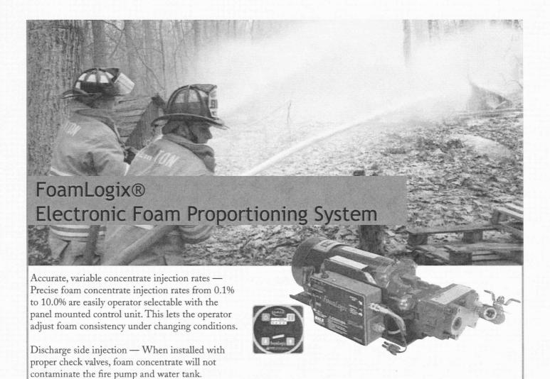
Push button automatic foam proportioning — Foam proportioning is fully automatic and water flow compensating.
